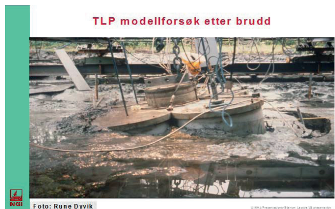
Figure 8.7. TLP model after failure (photo by Rune Dyvik, NGI).
