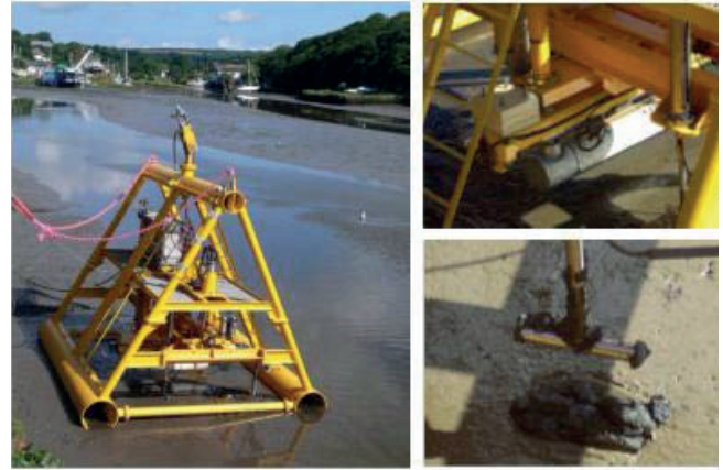
Figure 7.7. Pipe model tester (from Hill and Jacob, 2008).
