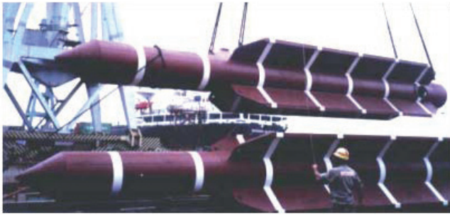
Figure 4.8. Photo of torpedo anchors used in the Albacora Leste Field, Brazil, in water depth up to 1384m (Brandao et al. , 2006).
